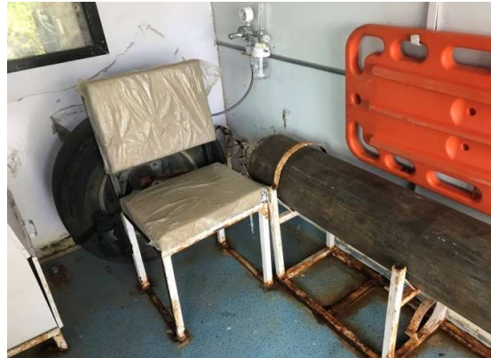
Tyre inside the vehicle and rusted stand
